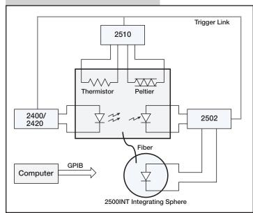
The Model 2502 is designed for tight integration with other Keithley instruments that are often used in LIV test systems for laser diode modules. These other instruments include the Model 2400 SourceMeter and Model 2510 TEC SourceMeter instruments.
